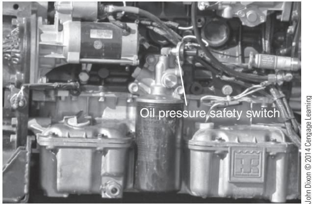
Figure 16-27 The oil pressure safety switch located in the oil filter housing; this switch stops the engine from running if engine oil pressure is lost, thereby preventing complete engine failure.
