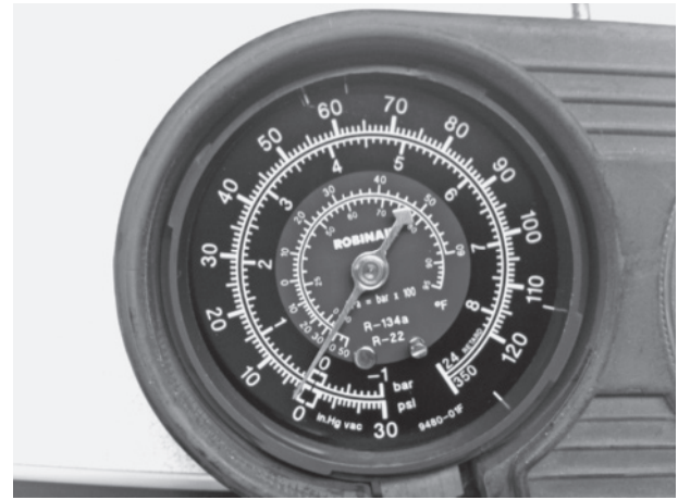
Figure 3-12 Manifold compound gauge reads both positive pressure and vacuum.
