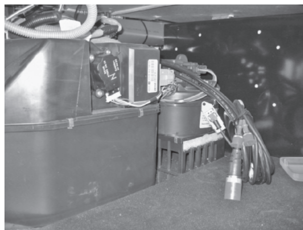
Figure 9-16 A bunk HVAC system containing the evaporator, heater core, blower fan, and ducting.
