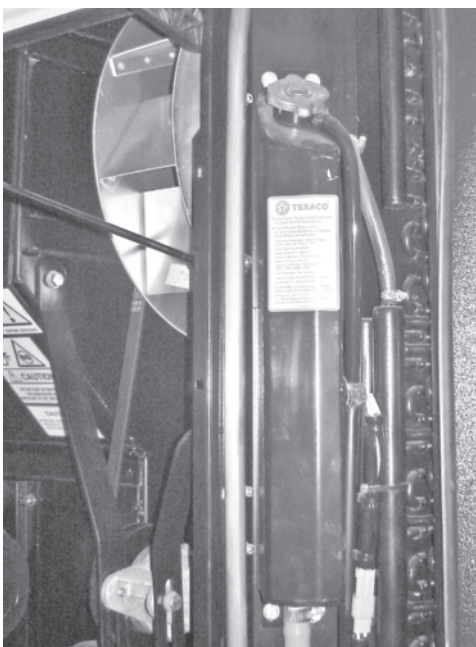
Figure 17-9 The coolant expansion tank with cooling system pressure cap.
