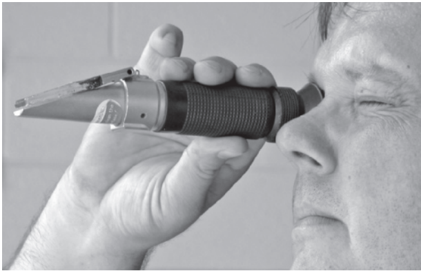
Figure 16-10 The correct method of using a refractometer to get a specific gravity reading of the electrolyte.
