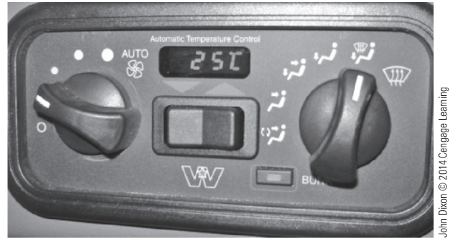
Figure 9-24 A control panel from a Western Star truck; the temperature display has been changed from degrees Fahrenheit to degrees Celsius.
