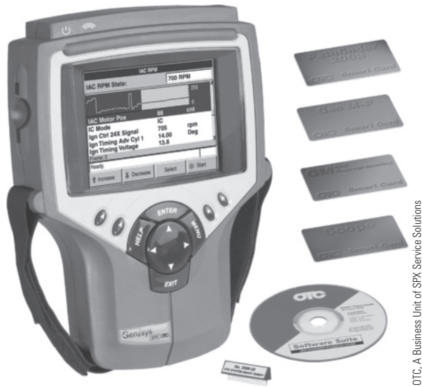
Figure 1-21 A scan tool; pictured is a ProLink 2000, used to improve the technician's trouble-shooting capabilities. HVAC system faults can be displayed on the reader. ProLink Web site.
