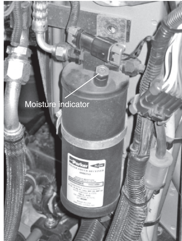
Figure 4-24 A receiver-drier containing a moisture indicator.
