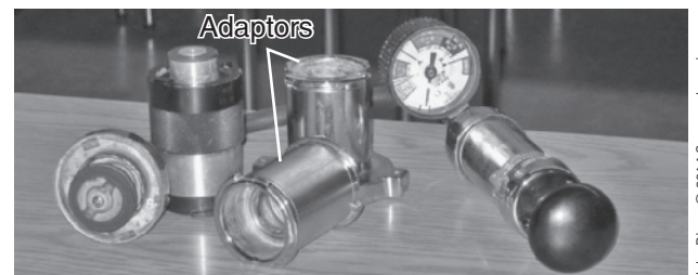
Figure 8-19 Pressure tester and adaptors for testing radiator caps.
