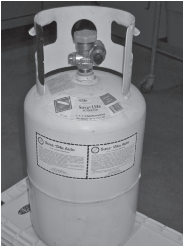
Figure 7-38 Refrigerant cylinder with one or two outlet valves.
