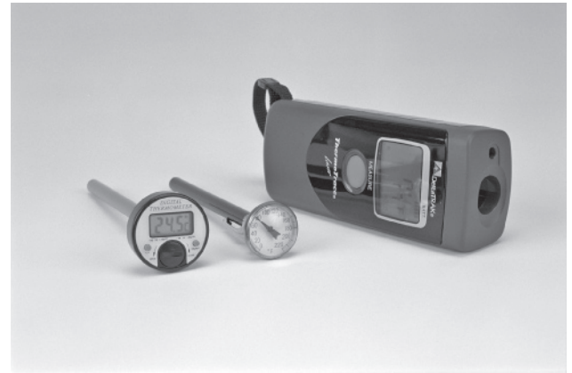
Figure 1-16 Thermometers are used by technicians to make accurate diagnoses of air-conditioning systems; shown are a few examples of temperature measuring devices.
