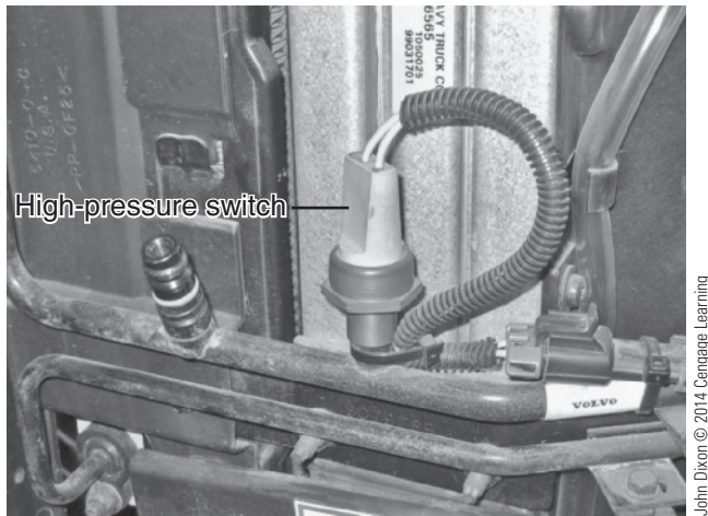
Figure 6-14 The high-pressure switch turns off the compressor when system pressure becomes too high.
