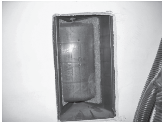
Figure 9-12 The recirculation door is closed, preventing dust and contaminants from entering the cab as well as reducing cooling time when air conditioning has been selected.
