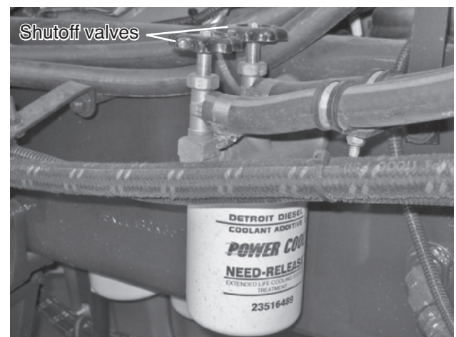
Figure 8-9 A typical engine coolant filter with hand shutoff valves.
