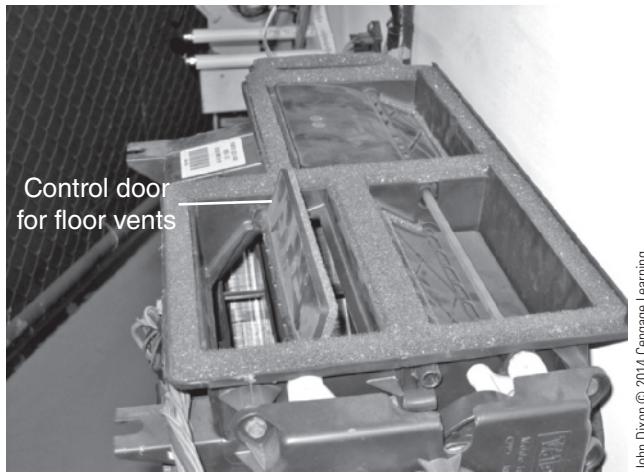
Figure 9-7 The vent door is open to direct air to the floor vents.
