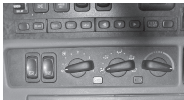
Figure 8-23 The dash controls for climate control of the truck cab.
