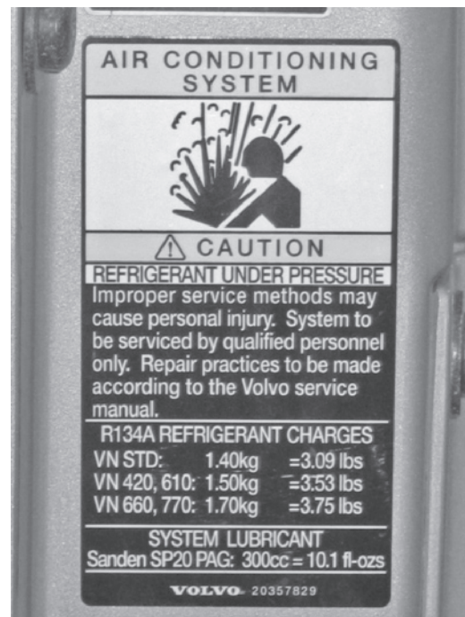
Figure 4-25 A warning decal on the firewall of a tractor that also lists refrigerant type and charge weight.
