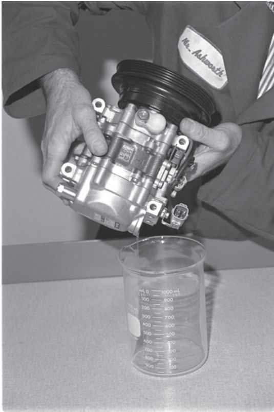
Figure 4-19 Checking compressor oil in a new compressor.
