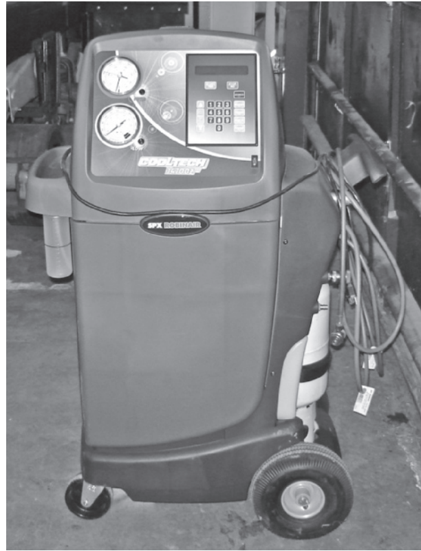
Figure 17-13 A refrigerant management center capable of performing all refrigeration-related servicing.
