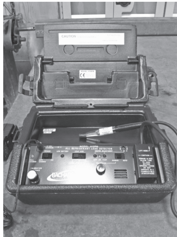
Figure 1-14 Electronic refrigerant leak detector for finding very small leaks.
