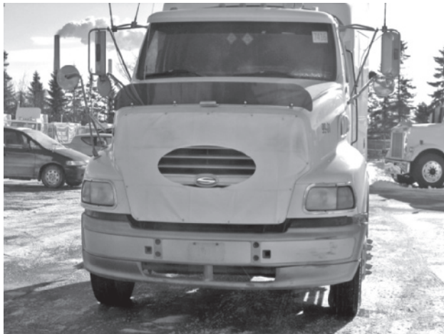
Figure 8-30 The winter front limits the amount of ram air that can be driven through the radiator and engine compartment.
