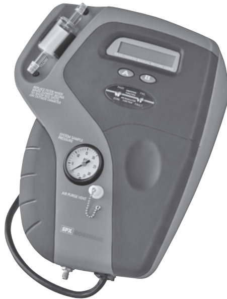
Figure 7-33 A refrigerant identifier, used to test the type and purity of refrigerant within the system.
