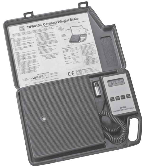
Figure 7-39 A refrigerant weigh scale, used to weigh in the correct amount of refrigerant.
