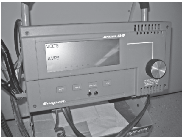
Figure 16-21 A tester used to load test batteries, starters, and alternators.
