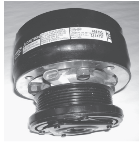
Figure 4-14 A typical scotch yoke, sometimes referred to as an R4.
