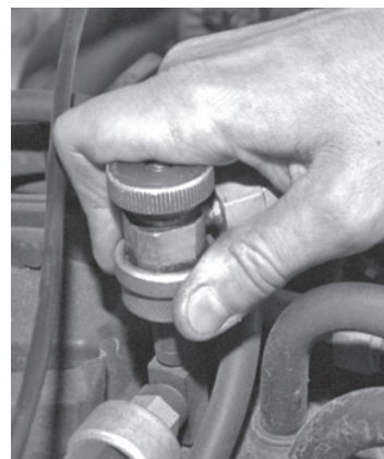
Figure 7-25 A manifold gauge hose end for R-134a systems.
